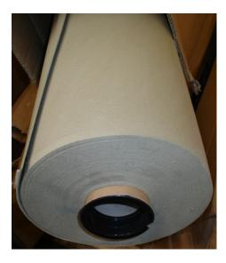
Refractory Mineral Fibre Paper
