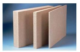
Vermiculite HD 1200 boards are based on the well known mineral Vermiculite, which is related to mica. Mixed with different binders and shaped under high pressure this product is used in all refractory applications, where high mechanical strength in combination with low thermal conductivity is asked for.
